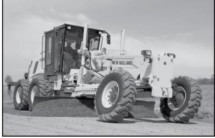
Featuring thin corner posts and door-With heavy-duty, box-section con- frames, and more than 62sf of glass area, the cab on New Holland motor graders provides an excellent view in all directions. An integrated sunshade reduces glare, and standard front and rear windshield wipers/ washers ensure a clear view. Interior and exterior mirrors help the operator keep tabs on any activity behind the machine.
