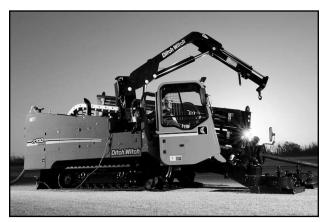
Ditch Witch's most powerful directional drill, the JT100 Mach 1 is equipped with a 268-hp engine.
