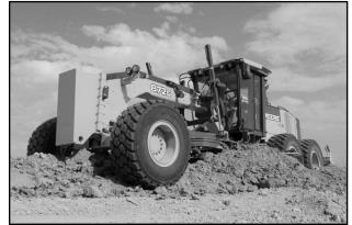
John Deere's G-Series motor graders offer users a choice of console-mounted standard controls or arm-rest-mounted standard fingertip controls, as well as features like cross slope control, automatic differential lock and a rearview camera.
