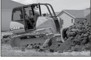
the 650L to work around low overhangs, while its lighter weight is ideal for work in soft soil conditions. The shorter track means easier turning, making the machine extremely maneuverable on the job site. The compact size also makes the crawler dozer easy to transport from job to job.
