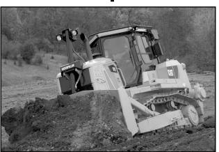
The Cat D7E Track-Type Tractor uses an electric drive system that delivers 10 to 30 percent greater fuel economy, greater productivity and lower lifetime service costs, compared with conventionally designed crawler tractors of equal weight and horsepower.
